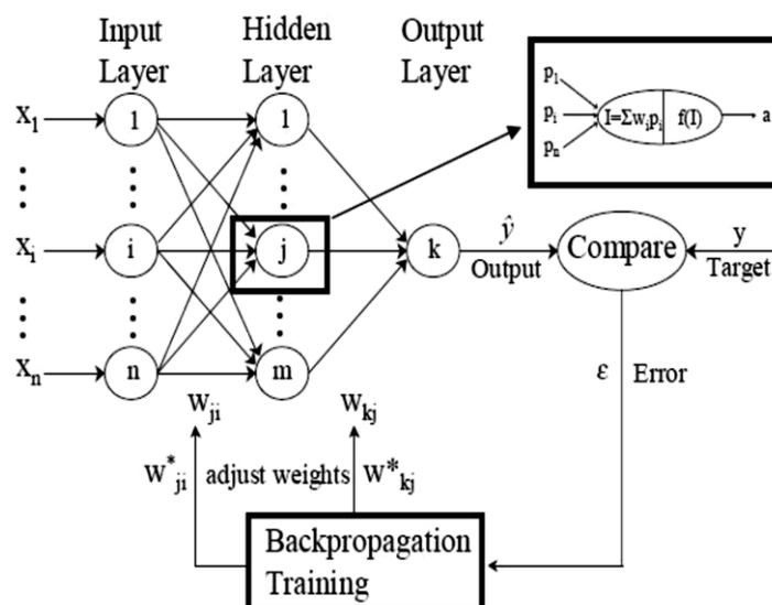
Figure 5: The Three-layer Neural Network with Back-Propagation (BP) Training Algorithm
